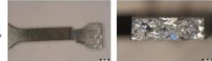
Fig. 6.12-6.16. The macrostructural aspects of the tensile fracture surfaces of the ZnCu alloy specimens
