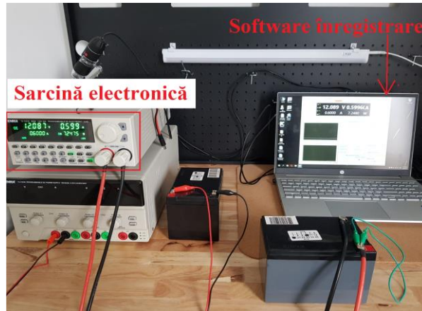
Fig. 5.2. Experimental assembly used to carry out the constant current discharge test
