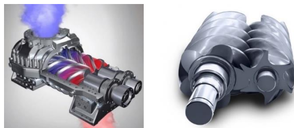
Figure 3. Screw compressor: design and principle (left) [15]; b) intermeshed rotors (right) [16]
