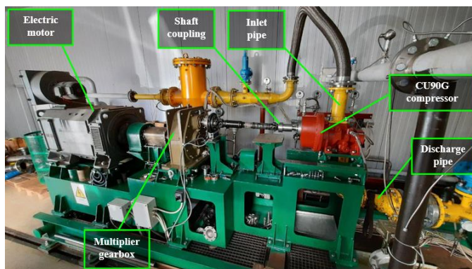
Figure 4. Compressor test bench
