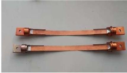
Fig. 19. HTS conductors without casing, made with the thermostated plate.
