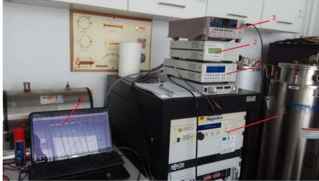
Fig. 27. The measurement chain used to test the HTS electromagnet.
