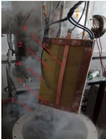
Fig. 17. 12 mm HTS tape junctioned, mounted on the testing support plate.
