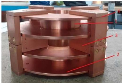
Fig. 15. Mechanical support of the HTS electromagnet.
