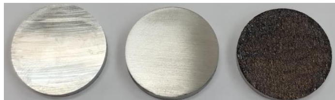
Figure. 7.3. The stages of the actual coating with CoCrMoNbTi HEA where on the left is the raw substrate, in the middle the prepared substrate and on the right the substrate covered by the ESD technique
