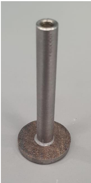
Figure 8.3. Clamping rod fixed with adhesive to the tested specimen
