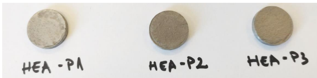
Figure 6.4. Macroscopic images of sintered HEA samples obtained by varying the temperature parameter
