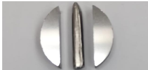
Figure 7.1. Electrode prepared for ESD deposition
