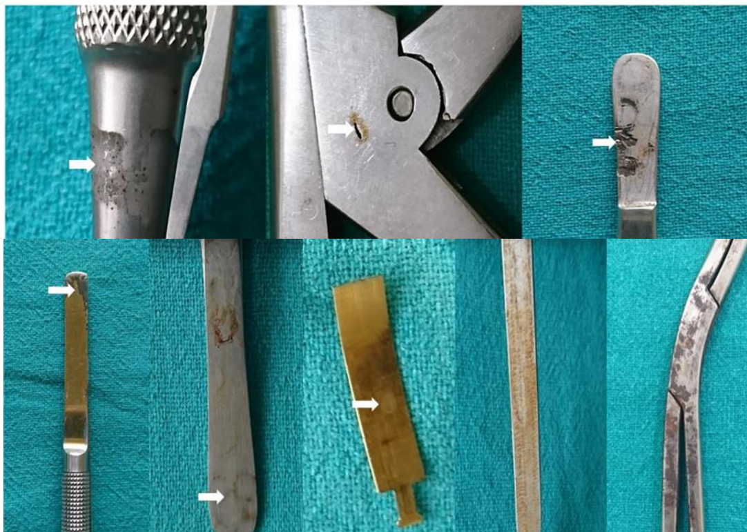
Figure 1.1. Corrosion effects on medical instruments. Images belong to Munakomi S, Shah R and Shrestha S. 2018, 7:102 [1.3]
