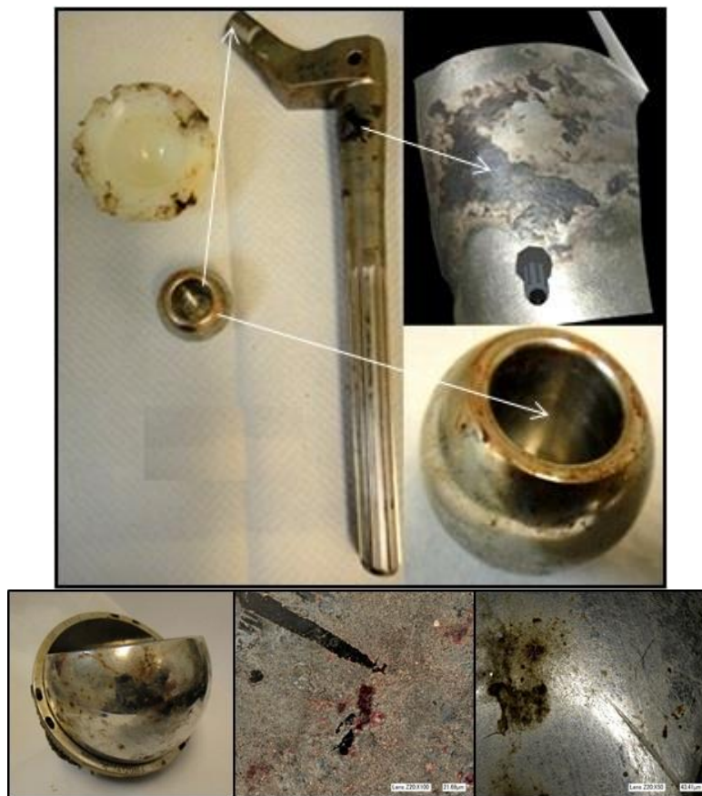
Figure 1.2. Corrosion effects in the case of implantable components. Images belong to The BONE Lab (Biomaterials for Osseointegration and Novel Engineering) 2024
