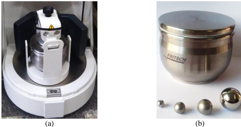
Figura 5.1. Fritsch® Pulverisette 6 Classic Line a) planetary mill and b) Stainless steel vial and balls.
