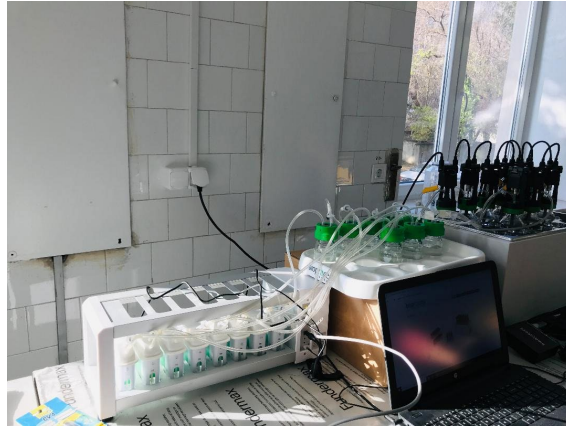
Fig. 5.7. Anaerobic digestion - laboratory scale experiment[68]
