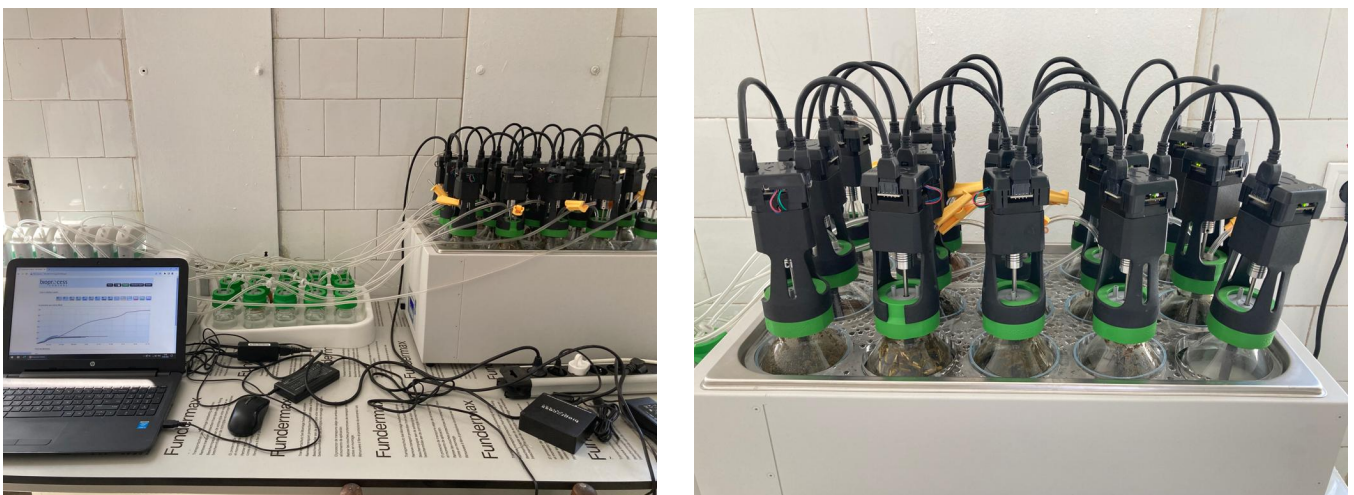
Fig. 5.2. Optimum mixtures of animal manure and agro-food by-products to obtain biogas using Gas Endeavour
