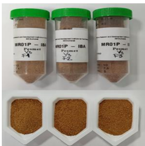
V3 (170°C, 180 minutes, 355 \mu\text{m} < D < 1000 \mu\text{m} )
