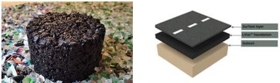
Fig. 5.1. (a): Cylindrical Littar® test sample – (b): Littar® in an optimal road structure – adapted from [66]
