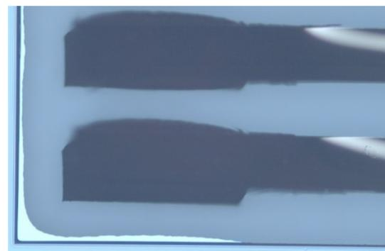
**Fig. 4.26.** Fully-released structures on silicon standard wafers
