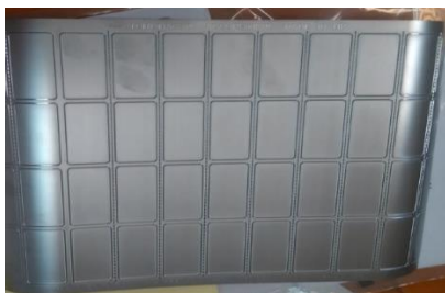
Fig. 2.1. Geometry of a die-cut for rectangular self-adhesive labels [31].
