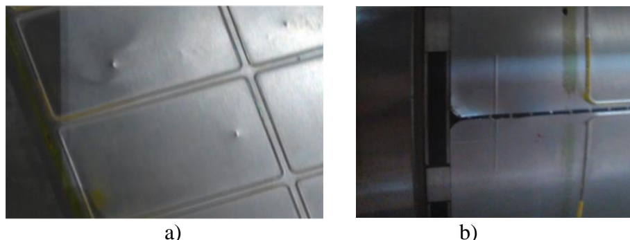
Fig. 2.14. Examples of mechanically damaged die-cuts: a) the surface of the plate is punctured; b) the bent corner does not adhere to the magnetic cylinder [37].
