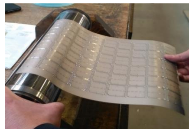
Fig. 2.2. Mounting the die-cut on the magnetic cylinder by rotating it [31].
