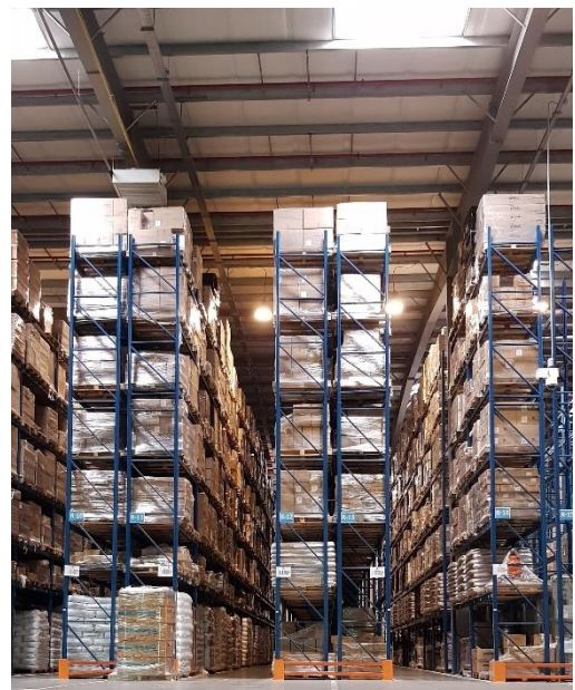
Fig. 1.2. Selective shelving systems. Photo source – Eurocoper S.A.
