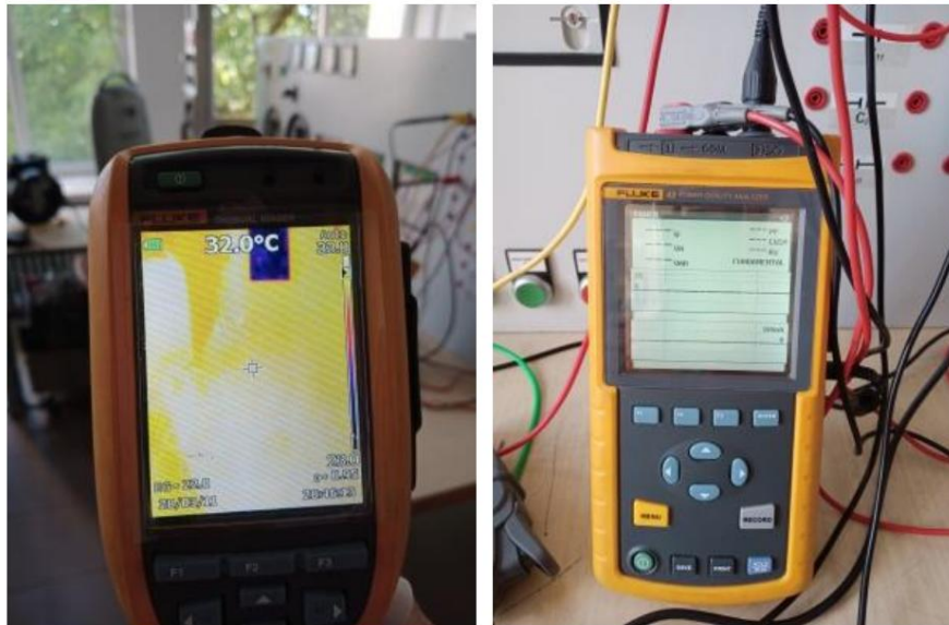
Fig. 12 Conductor temperature after 15 min. from the passage of the electric current.
