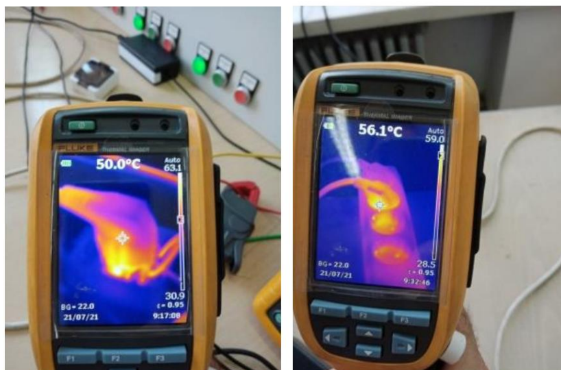
Fig. 16 Temperature at the contact points after approx. 30 minutes from the beginning of the experiment.
