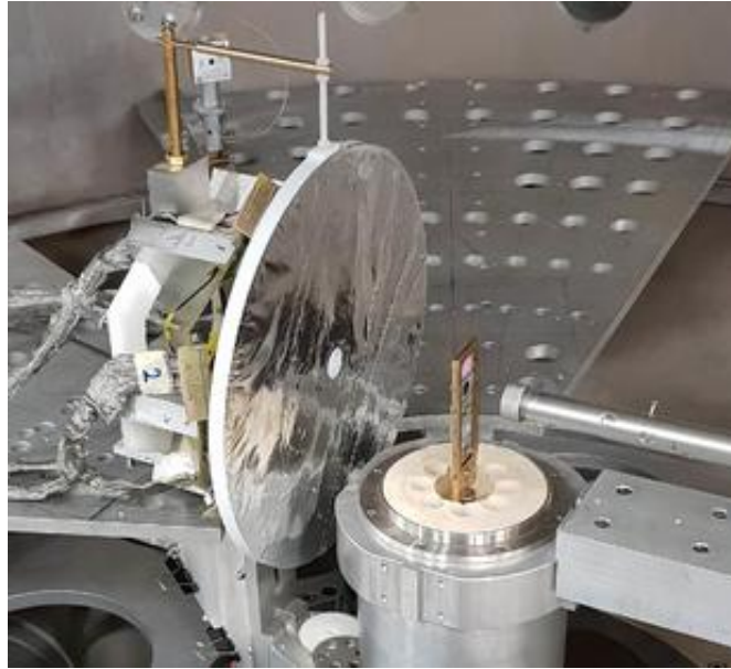
Figure 4.3 LHASA - the experimental set-up used for the study of ^{19}\text{F}(p,\alpha)^{16}\text{O} reaction cross section.
