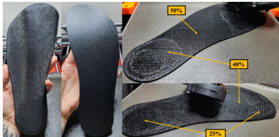
Fig.6.8. Filaflex 60A, left foot insole (25%, 40%, and 50% infill)
