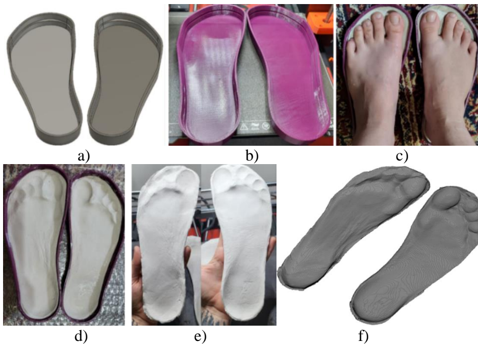
Fig.6.5. Evaluation of maximum plantar pressure: a) 3D modeling of the molds; b) 3D-printed molds; c) clay formation; d) clay curing shapes; e) hardened clay; f) scans of the foot imprints.
