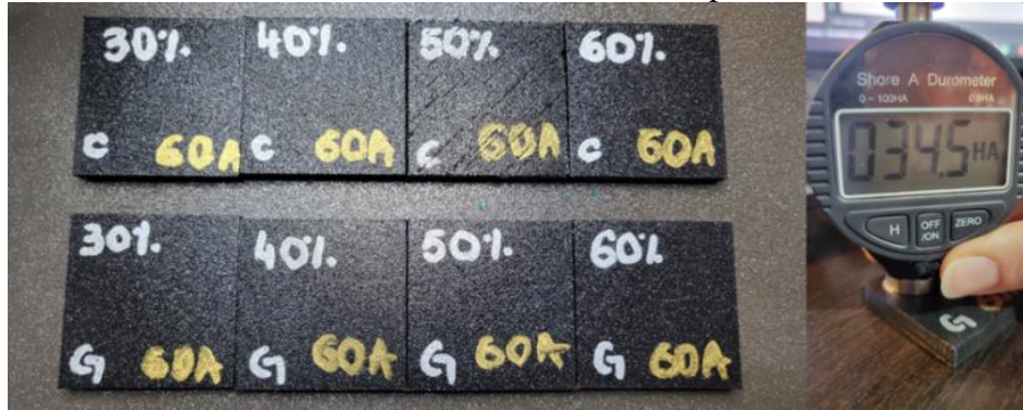
Fig.6.6. Filaflex 60A – specimens and measurement with shore A durometer
