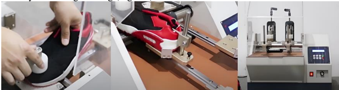
Fig.3.2. GT-KA01-2B Footwear durability testing machine [76]
