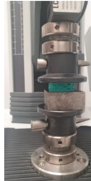
Fig.7.18. Compression testing of a varioShore TPU specimen
