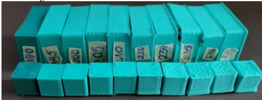
Fig.7.3. Material flow calibration tests
