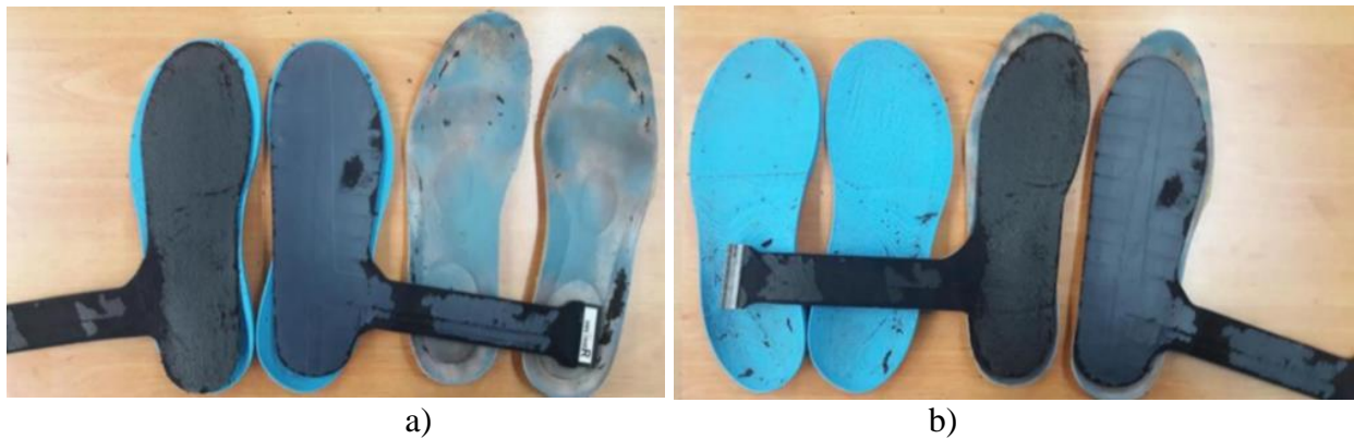
Fig.7.7. In-Shoe Pedar pressure measurement system: a) 3D printed blue Filaflex 82A insoles (left); b) Original shoe insoles (right).
