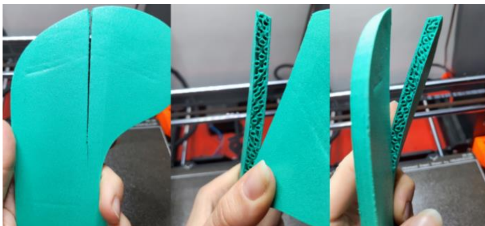
Fig.7.10. The insole varioShore 1 show no degradation of the internal structure.
