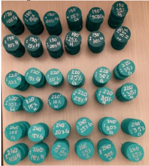
Fig.7.17. Samples prepared for compression test
