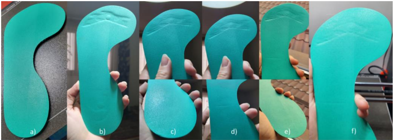
Fig.7.11. The evolution varioShore 1 insole after: a) 3D printing; b) 7,000 cycles; c) 42,000 cycles; d) 63,000 cycles; e) 98,000 cycles; f) 48 hours after testing.
