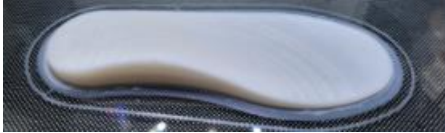
Fig.5.4. Insole made of PCL
