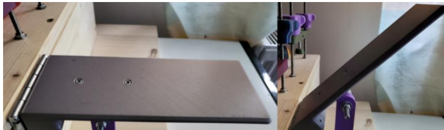
Fig.3.12. Support surface at 0° and at 45° relative to the support plane.
