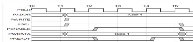
Figure 3.6. APB Write transaction waveforms (ARM, 2023)
