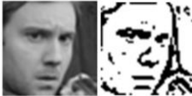
Figure 4.8 Applying the Adaptive Thresh Gaussian Filer to a photo
