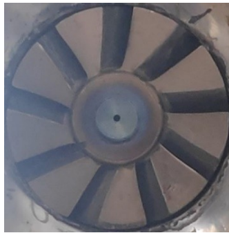
Figure 2.9- The Swirl injector with central orifice 2 mm in diameter for fuel injection into the combustion chamber.
