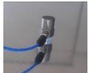
Fig. 8.18. Mounting the accelerometer on the experimental model of the carbody.
