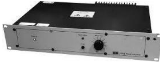
Fig. 8.14. Amplifier LDS PA25E.
