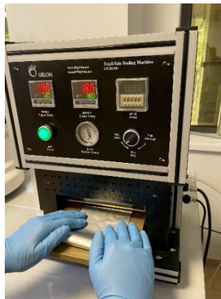
Fig. 12. System for manufacturing casings for pouch cells
