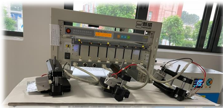
Fig. 18. Testing of pouch cells on the testing system
