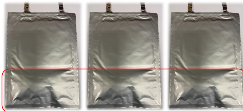
Fig. 19. Multi-layer pouch cells NMC811/graphite after formation
