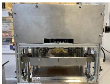
Fig. 10. The profile system used in the production of electrodes
