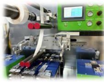
Fig. 11. Semi-automatic assembly system for pouch cells
