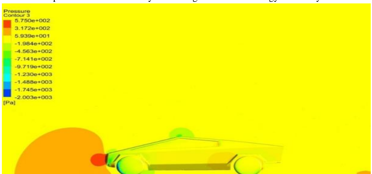
Figura 4.1 Digital simulation for pressure analysis
