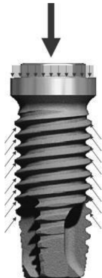
Figure 1.12. Axial load distribution. The morphology of the threads can influence the nature of the compressive force created in the bone surrounding a machined implant. [1]
