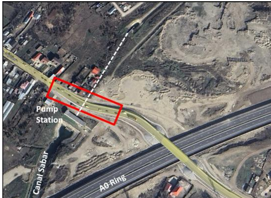
Figure 10.1. Location of the roadway ramp in relation to the municipal pipeline and the positioning of the Pumping Station relative to the A0 Highway; the dotted white line indicates the pipeline located beneath the embankment, surfacing a few meters further on
