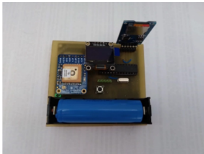
Fig. 4.2 The electronic module in the final version - top view
