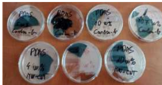
Fig. 4. 1 PDMS-MWCNTs nanocomposite samples made with different amounts of MWCNTs (4% wt, 7% wt and 10% wt) and Carbon black (5% wt, 7% wt, 10% wt and 10.7% wt).
