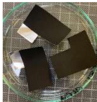
Fig. 7. 3 90% Activated Carbon and 10% PVDF electrodes deposited on aluminum manifold, cut to size 4.5x2.5 cm (11.25 cm 2 )
