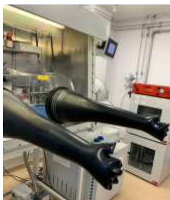
Fig. 6. 1 The Glove-Box inside which the cells were safely assembled
