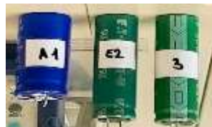
Fig. 3. 6 The 3 commercial supercapacitors from 3 different manufacturers available of 100F and 2.7V: A1, E2, code 3.
