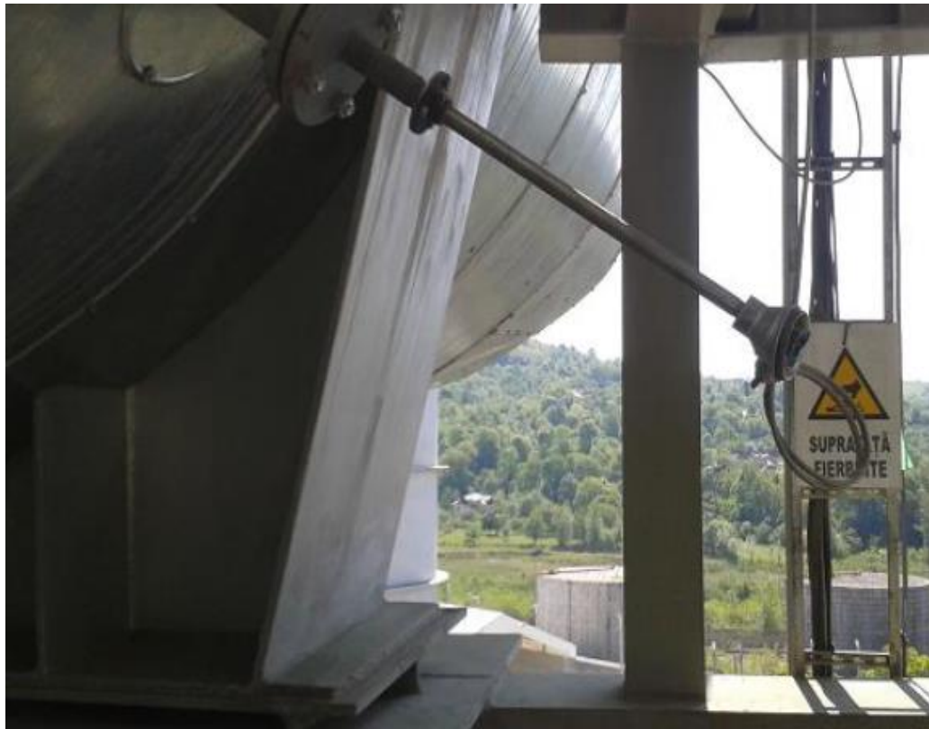
Figure 5.23. Installation place of the intelligent temperature sensor at the cement factory
