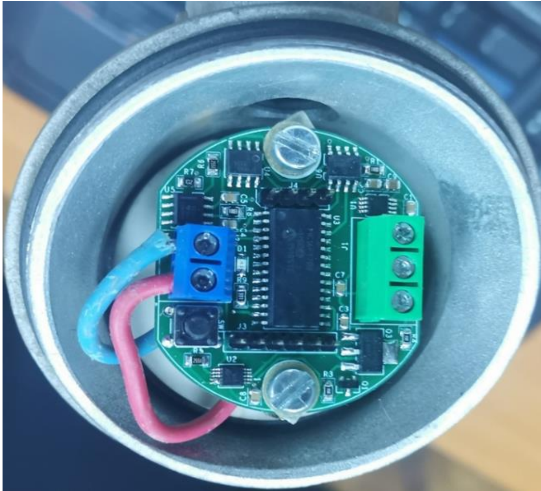
Figure 5.15. Placement of the circuit inside the sheath of a temperature probe used in a cement factory
