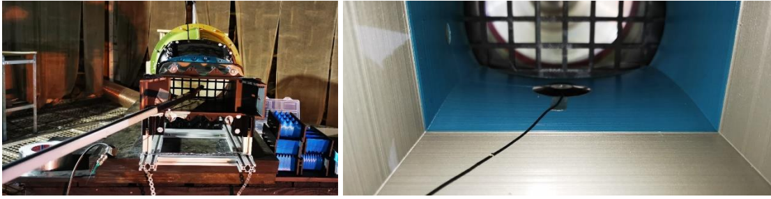
Figure 21. Microphones placement for identifying turbulence parameters (left – aerodynamically profiled microphone, right – surface-mounted microphone)
