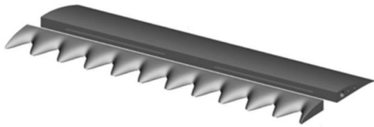
(c) 3D printing modular serrated LE edge [7]
